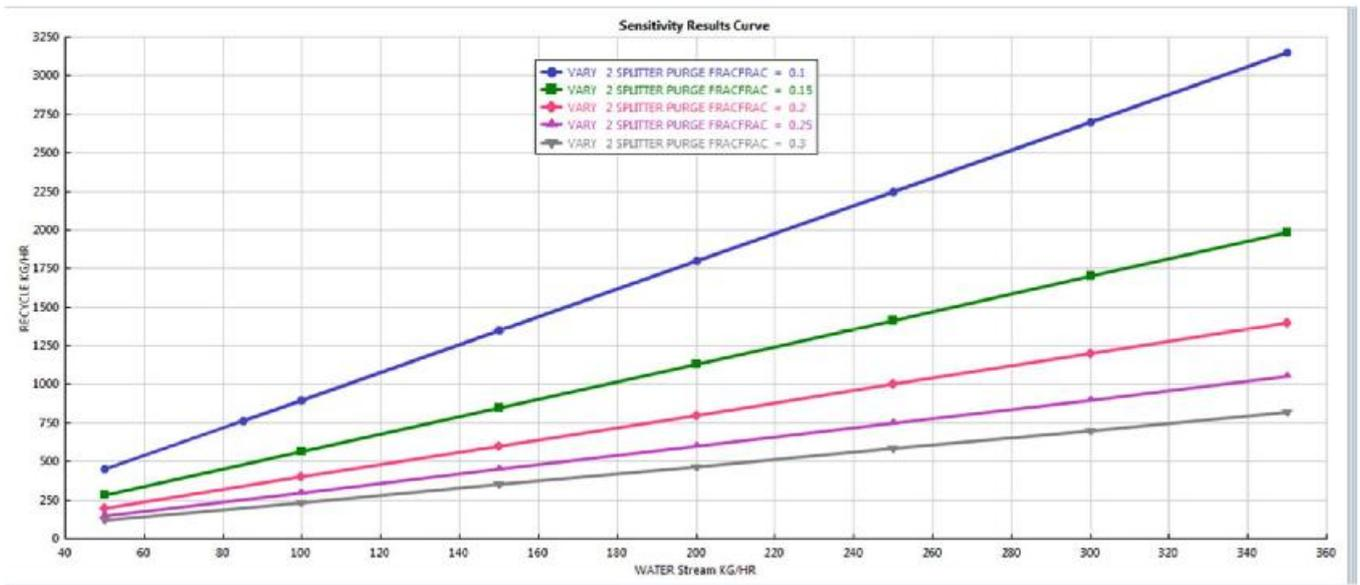
Figure 6 shows that the minimum required water make-up flow of 250 kg/h has an associated recycle flowrate of approx 600 – 2250 kg/h. As can be seen, a high splitter purge fraction of 0.3 results in the minimum recycle of 600 kg/h. This is for a biogas mass flowrate of 5.86 kg/h.
