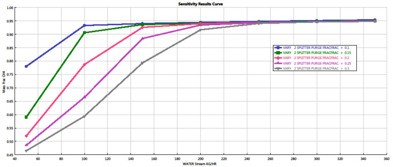
It can be seen from Figure 5 that a high water make-up rate ( $\geq 250$  kg/h) is required to avoid build-up of impurities in the recycle stream, to achieve the required upgraded biogas specification of 95% CH<sub>4</sub>.
