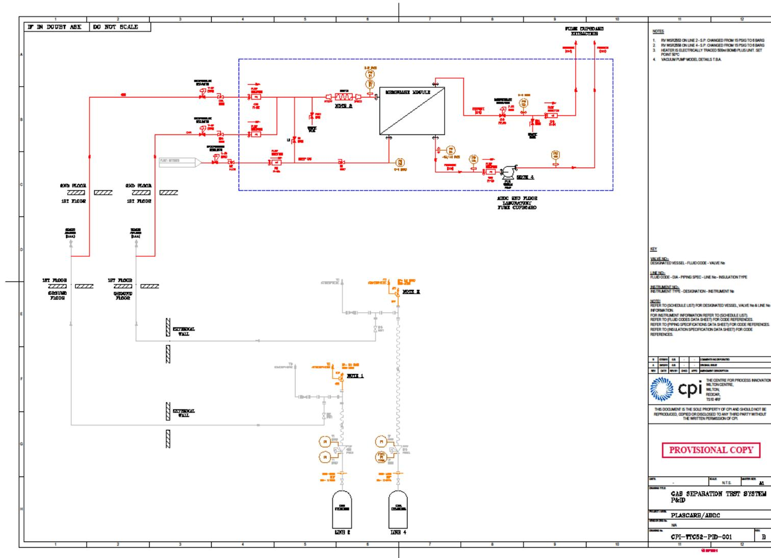
Figure 8 P&ID of Laboratory scale membrane unit and feed streams.
